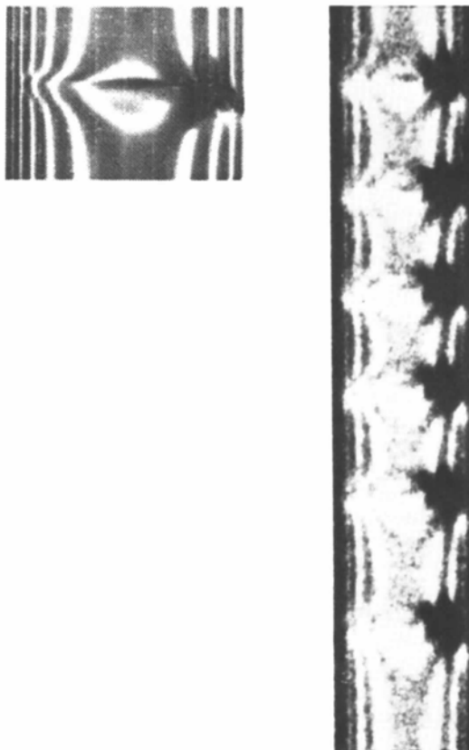
Fig. 2. Section topograph of a silicon wafer, Mo K\alpha , 333.
